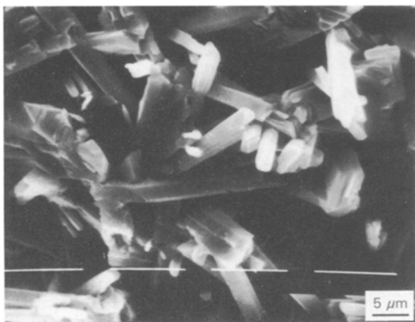
Figure 5 Scanning electron micrograph of the set plaster from \alpha -hemihydrate plus 2 wt% K 2 SO 4 ( w/s = 0.6 ).
