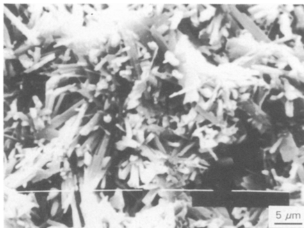
Figure 4 Scanning electron micrograph of the set plaster from \alpha -hemihydrate plus 2 wt % BDH (6.7 \mu\text{m} ) dihydrate ( w/s = 0.6 ).
