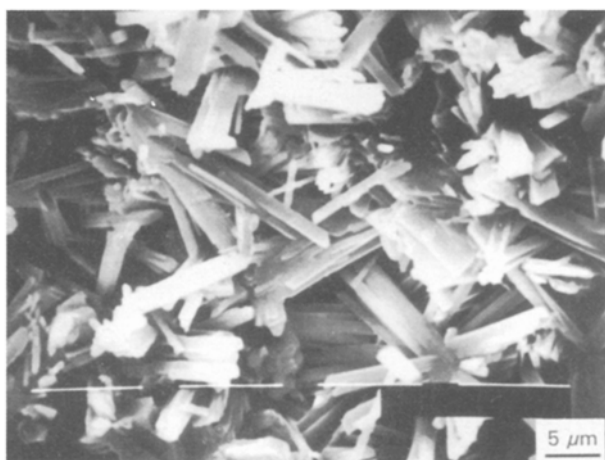
Figure 3 Scanning electron micrograph of the set plaster from \alpha -hemihydrate ( w/s = 0.6 ).
